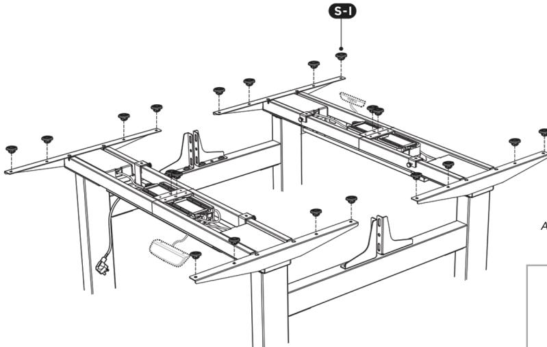
Attach the anti-vibration pads (S-I) to the surface of the crossbar on all twenty positions as shown.
