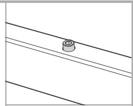
Loosen the hex head screws that fix the adjustable junction, but don't completely take out the screws.
