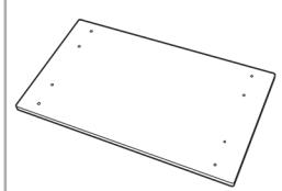
After tightening the screws, use a drill to make mounting holes on the backside of the tabletop through the 8 mounting holes on the side brackets.
